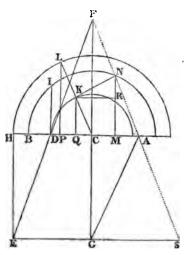
HD, which determines the greatest inclination of the thread; and at any subsequent part of the vibration, if the point of suspension be advanced from D to M, the time elapsed will be expressed by the arc IN, DI and MN being perpendicular to AB, and taking HL similar to IN, the perpendicular LP will show the place of the pendulous
